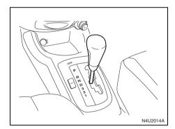
Movement between certain positions requires pushing the shift lever to the passenger side while shifting. This prevents you from changing positions unexpectedly
